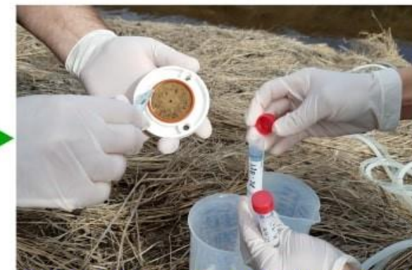
Filter folded and inserted into 15ml falcon tube with ATL buffer
