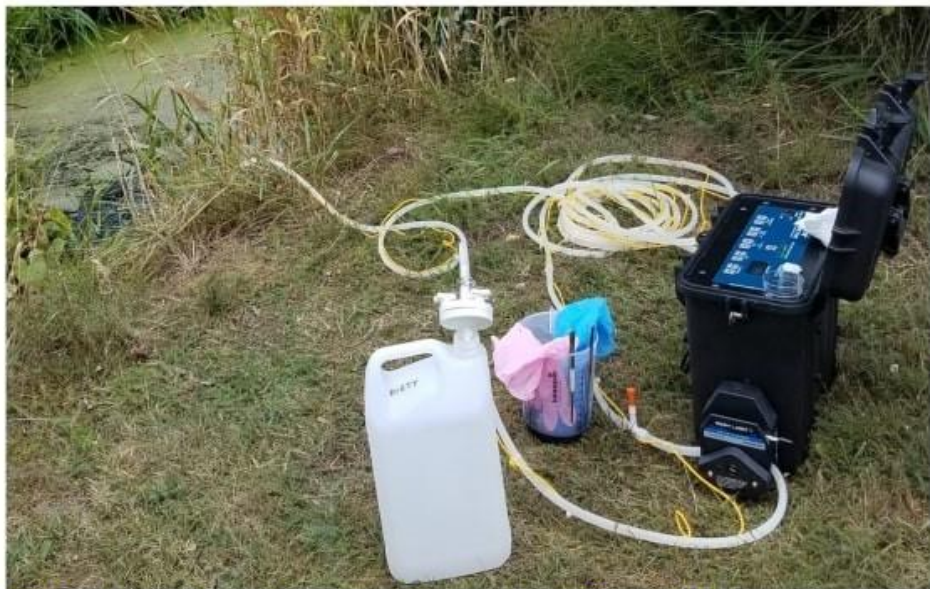
Filtration of water samples using Peristaltic pump, tubing, and the sampling vessel
